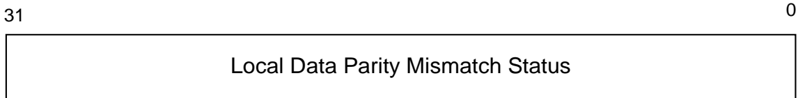
Figure 7-78: 16.0 GT/s Local Data Parity Mismatch Status Register
