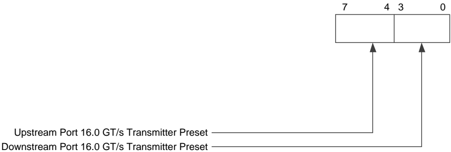
Figure 7-82: 16.0 GT/s Lane ((Maximum Link Width - 1):0) Equalization Control Register Entry
